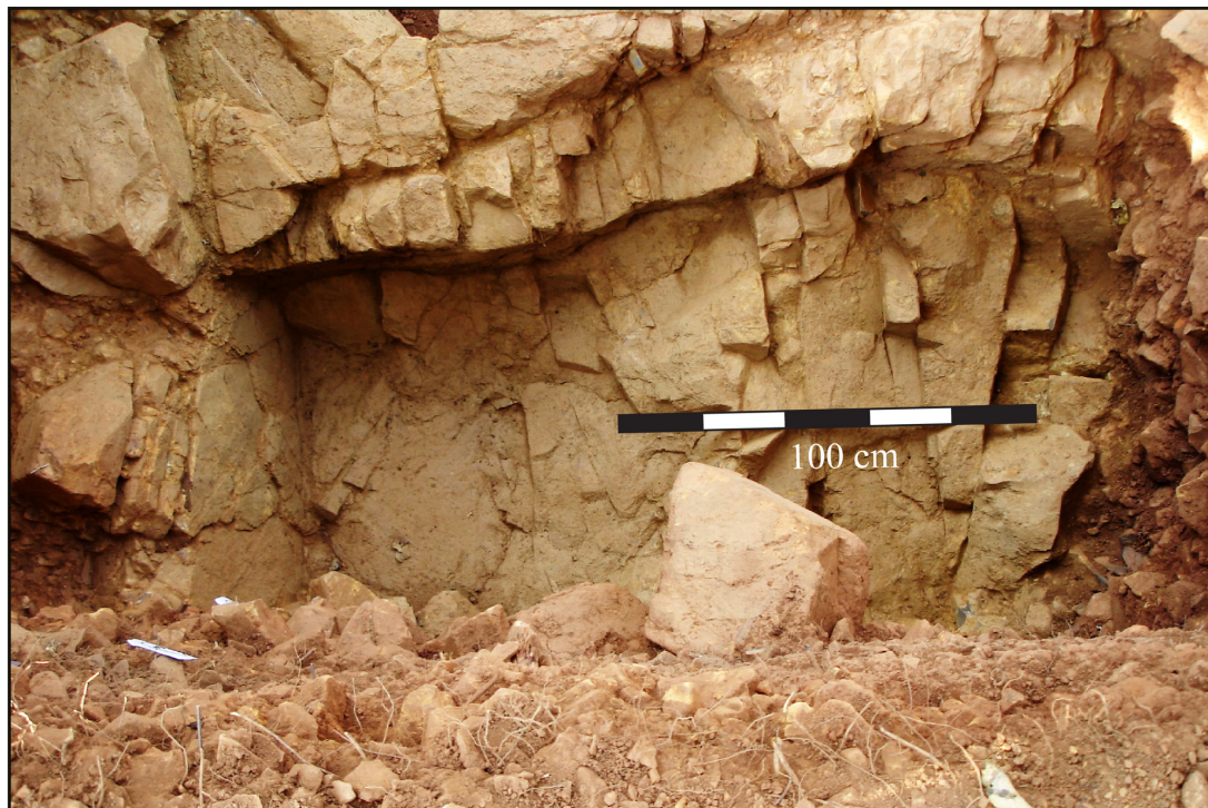
Figure 10: Showing the quarried blocks of highly jointed dolerite dyke, revealed during the section scraping at Mound-III of Sulabhdih.
